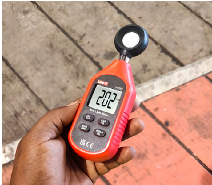
> Illumination of loading / unloading bay at Loghub
